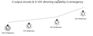
During a power outage, the emergency fixtures are dimmed to field selectable levels of 25%, 50% or 75% brightness output. Reducing wattage draw from the fixture will allow for more fixtures to be connected to the Mini Inverter, offering an extremely versatile solution for many applications.
