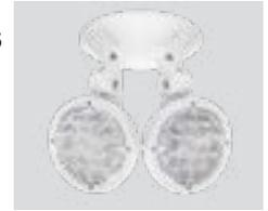
The Cluster™ LED ELF652D/LED Remote head can ONLY be powered from the UQLXN-2LED combo or LCA 2LED battery units of the same family. Used for internal or external applications, the indoor remote head draws 3.6V-3.6W and Weather-Proof head draws 3.6V-3.8W
